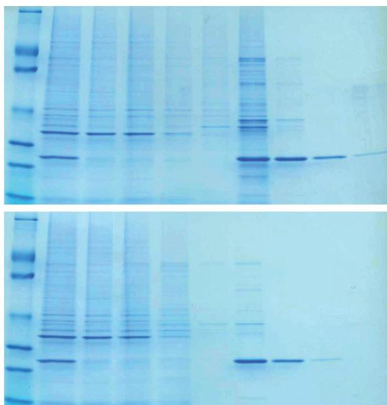
Figure 21: Bacteria expressing a His-tagged protein were lysed with Bacterial PE-LB™ and the recombinant protein was purified with HOOK™ 6X His Protein Purification kits (Top: Nickel resin; Bottom: Cobalt resin). Lane 1: PAGEmark™ protein ladder; 2: Cleared lysate; 3: Flow through; 4-6: Washes; 7-9: Elutions.
